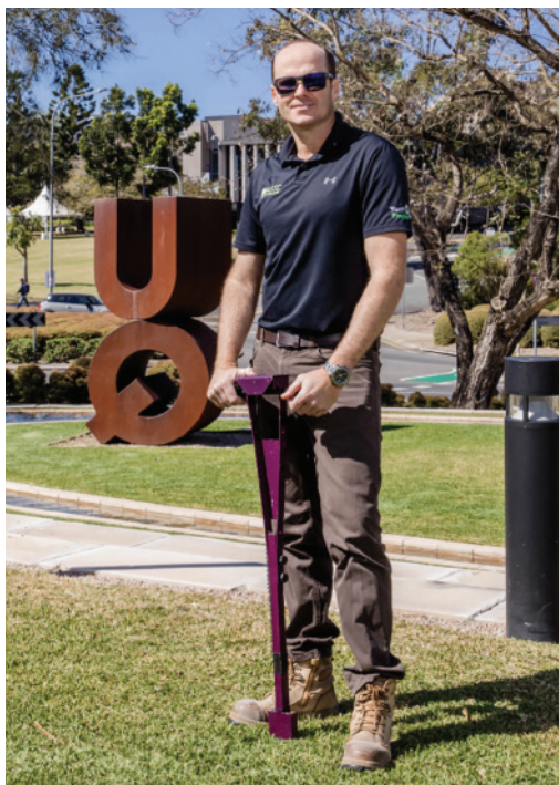
Above: Matt Roche using a 'soil moisture meter', which is used to measure the soil moisture content of the rootzone. Image: Anjanette Webb.
